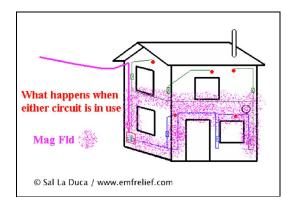
The magnetic field (when there is one) will exist and broadcast into free space regardless of the wire type. This shows a wiring error regarding lighting, which may be more common than for Power circuits. Nonetheless due to uncle Floyd and cousin Jack doing "creative wiring" over the years, any type (and mixture) of circuit can be involved.
