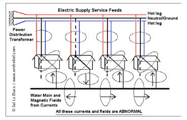
When several homes are fed from the same power transformer as above, even if the water pipe and electrical service are located on the same side of the house (an ideal situation that could reduce the wide-area impact of split neutral currents), a magnetic field may exist from water piping in the street that could negate any of the considerations presented here, in that even neutral isolation would not accomplish a substantial reduction of the magnetic field presence.
